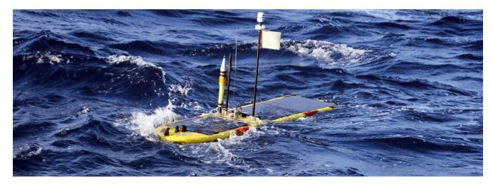
The NDSF Waveglider is the latest addition to the National Deep Submergence Facility's suite of tools, adopted after years of development. This cutting-edge surface vehicle, purchased through Liquid Robotics, can be used in conjunction with any NDSF vehicle or as a standalone tool.
