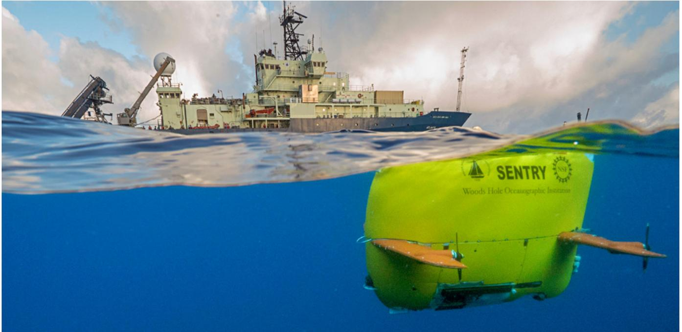
The autonomous underwater vehicle (AUV) Sentry is the newest member of the National Deep Submergence Facility having been adopted to replace its predecessor ABE in Summer 2010. Sentry is designed for operations down to 6,000 meters (19,685 feet) depth, with a design that emphasizes extreme maneuverability, close bottom following, large and innovative payloads, and rapid transit to and from the seafloor.
